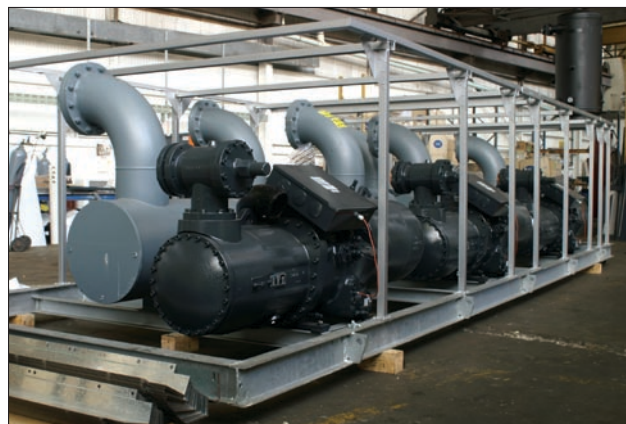
One of the new 750kW chillers sitting on its hot dip galvanised base.
